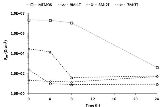
**Fig. 7.** Evolution of the pore resistance versus time of contact with electrolyte of the coatings MTMOS, 9M:1T, 8M:2T and 7M:3T.
