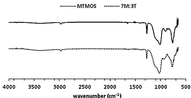
Fig. 2. FTIR spectra (region 4000–400  $\text{cm}^{-1}$ ) of MTMOS (a) and 7M:3T (b).
