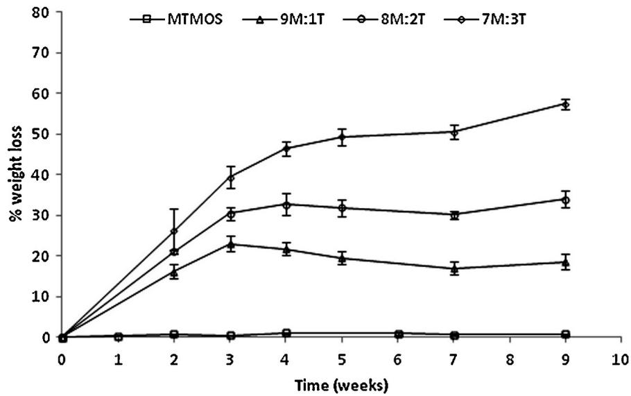
Fig. 3. Weight loss by hydrolytic degradation versus time of immersion in distilled water for MTMOS, 9M:1T, 8M:2T and 7M:3T coatings.
