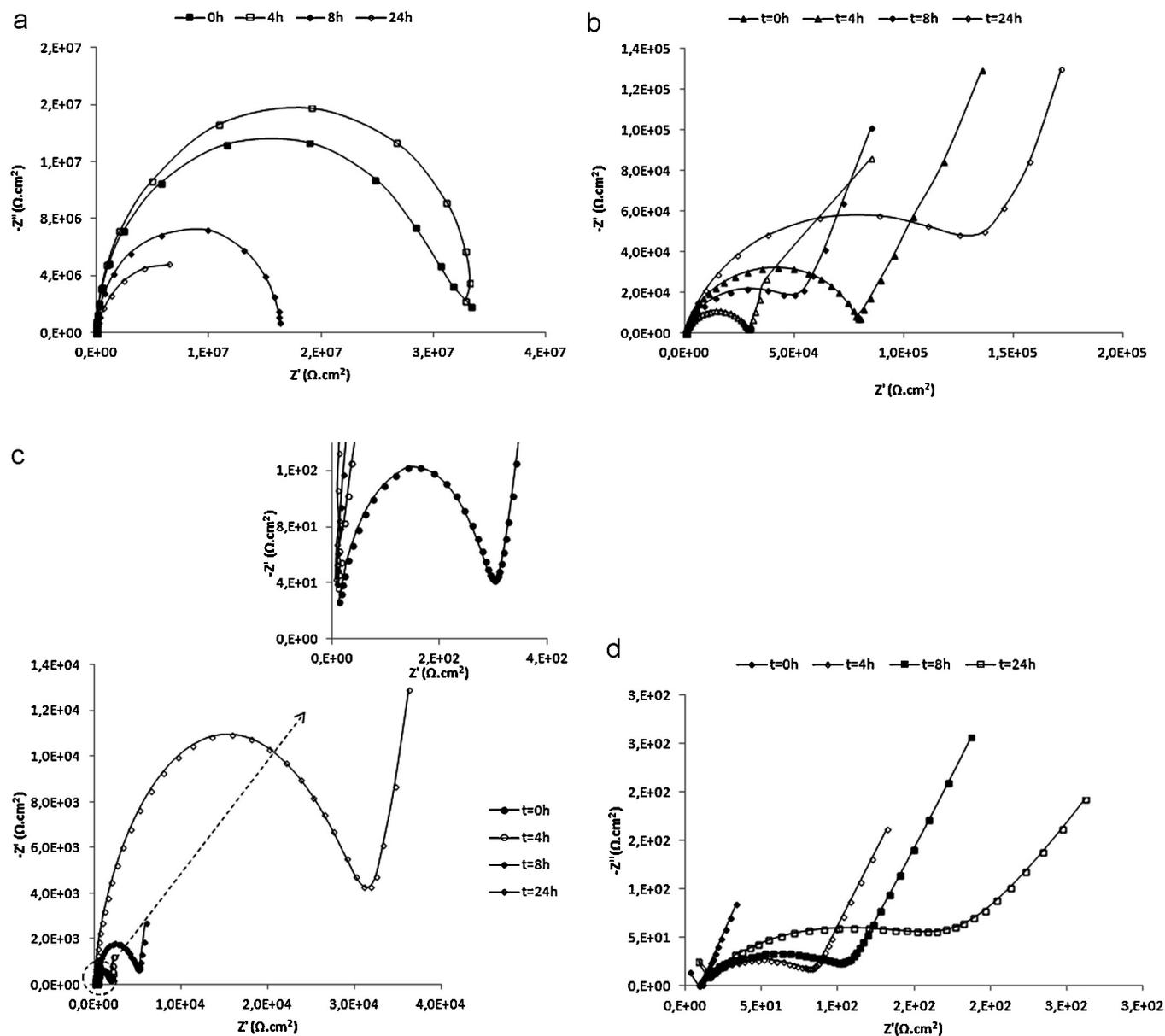
Fig. 5. Evolution of Nyquist plot for (a) MTMOS, (b) 7M:3T, (c) 8M:2T and (d) 7M:3T coatings during 24 h immersion in electrolyte (deionised water 3.5% NaCl by weight).
