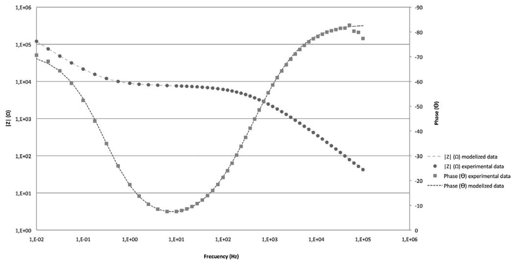
**Fig. 6.** Bode plot for 8M:2T sample after 10 h in contact with electrolyte. Comparison between experimental data and modelisation results with equivalent circuit.
